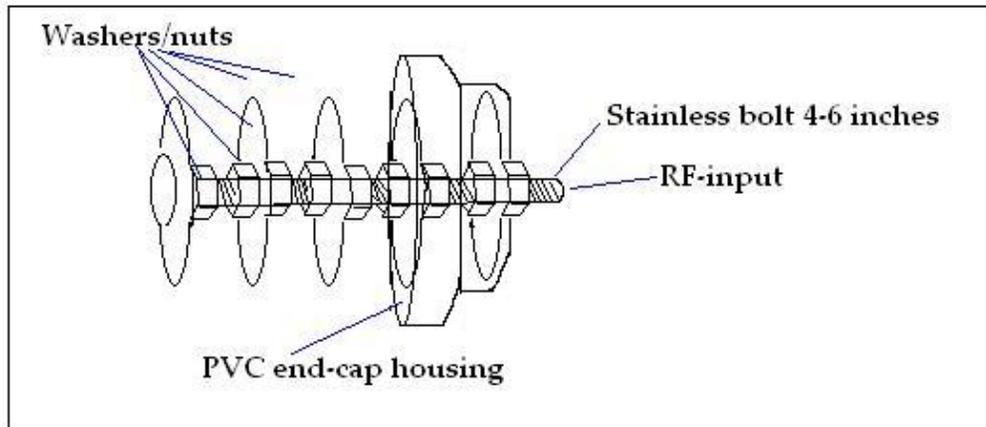
Fig. 1: IFA "Spaced-Washer Probe" Concept
