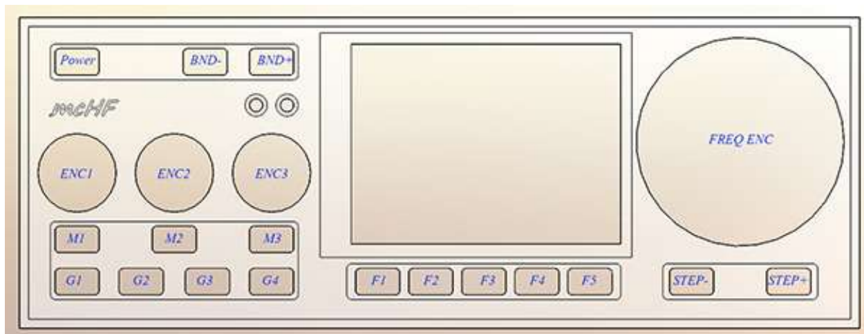
Figure 1: Front panel controls of the mcHF transceiver
