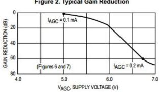
Figure 2. Typical Gain Reduction
