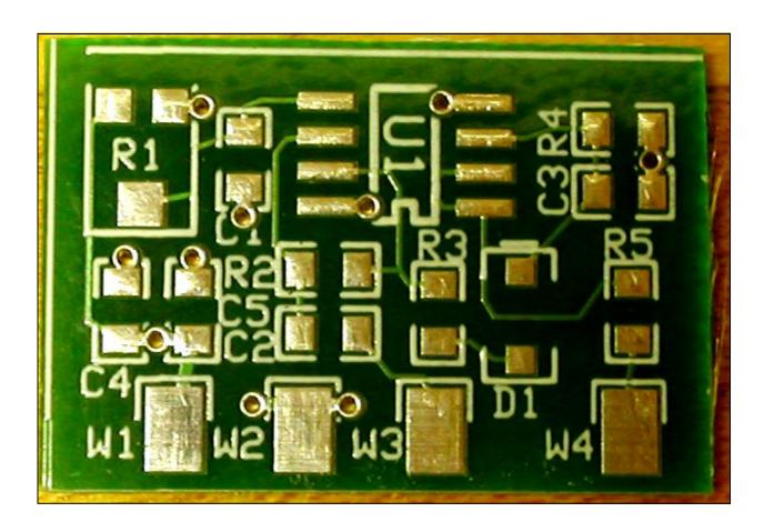
ONLY 2 COMPONENTS ARE POLARITY SENSITIVE – U1 AND D1. THE SMD PART U1 HAS A GRAY DASH ON THE END THAT DENOTES PIN 1. THAT GRAY DASH END OF U1 HAS TO CO-INCIDE WITH THE "NOTCH" ON THE SILKSCREEN OUTLINE OF THE PCB.
