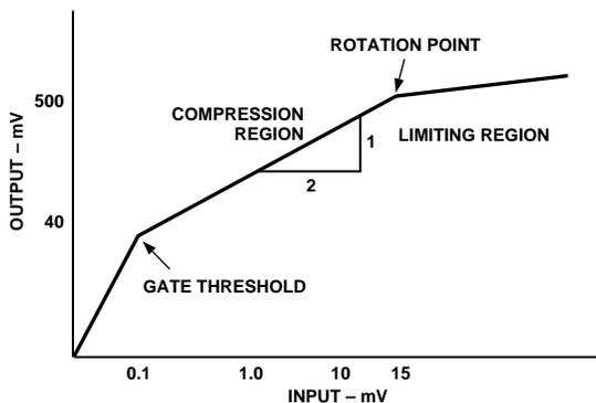
Figure 25. Transfer Characteristic
