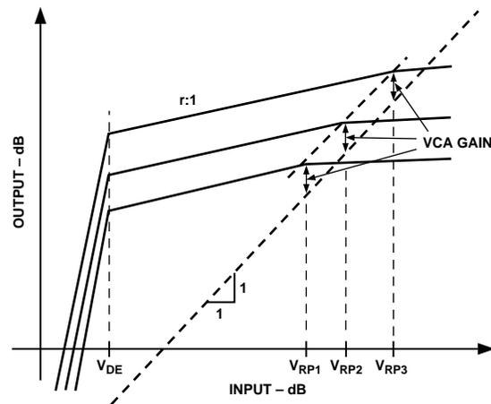
Figure 17. Effect of Varying the Rotation Point
