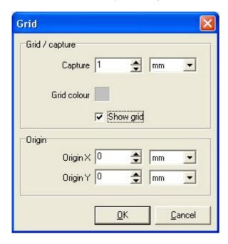
The capture is variable from 0.1 to 10 mm.
