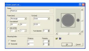
This function creates a <u>group</u> which contains the frame for the component dimensions and the cut for the component. Circles and rectangles are available as shapes for the frame and the cut. Mounting holes can be added if necessary. The distance of these holes is measured between the centres of the holes.
