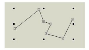
The corners of polygons, rectangles and lines (points) are marked with tiny rectangles as well, as long as one of these objects is selected. This allows you to move (drag and drop) points to another position. When the mouse cursor is moved on a point (cross cursor), a local popup menu (right mouse button) offers the functions DELETE POINT and ADD POINT.
