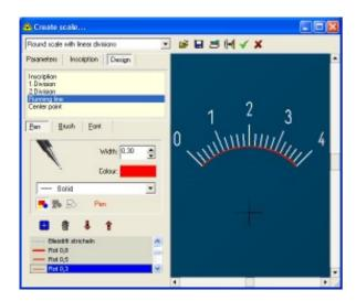
You can click on DESIGN to change <u>pen</u>, <u>brush</u> and <u>font</u> of the scale individually. A list shows the components of the current scale (1. Division, 2. Division, Centre point, etc.). This list is used to select the components that you want to modify. You can select one or more entries of the list. (To select more than one object, hold down SHIFT during selection.)
