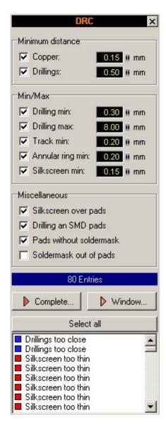
Here you can adjust the DRC-settings. You can also select or deselect single DRC-checks with the checkboxes.
