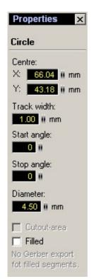
During the input of the diameter note that you must include the width of the drill. Since the tool will mill concentrically around the radius, the milled hole width will be wider. You must take the milling tool width off from the diameter of the hole, in order to obtain the correct hole width result. In our case we want a hole of 5,5mm and our milling tool has a width of 1mm. The input in the circular
