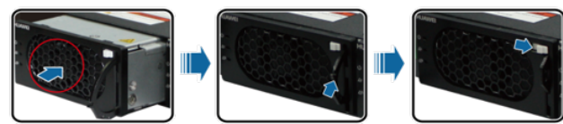
Figure 6 Installing a rectifier
