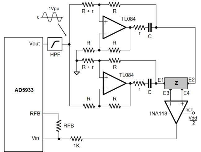
Fig. 3 Schematic of the Mirrored Howland-Modified Current Source
