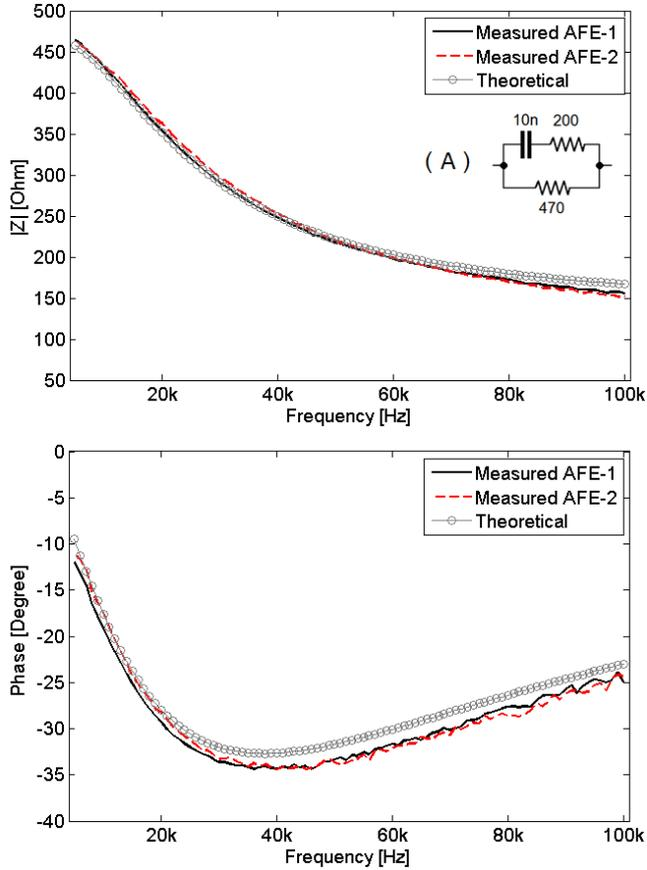
Fig. 4 Frequency response of both module and phase load impedance A.
