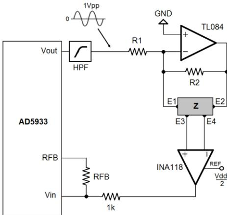
Fig. 2 Schematic of the Load-in-the-Loop Current Source
