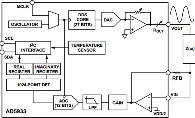
Fig. 1 AD5933 Functional Block Diagram [10]
