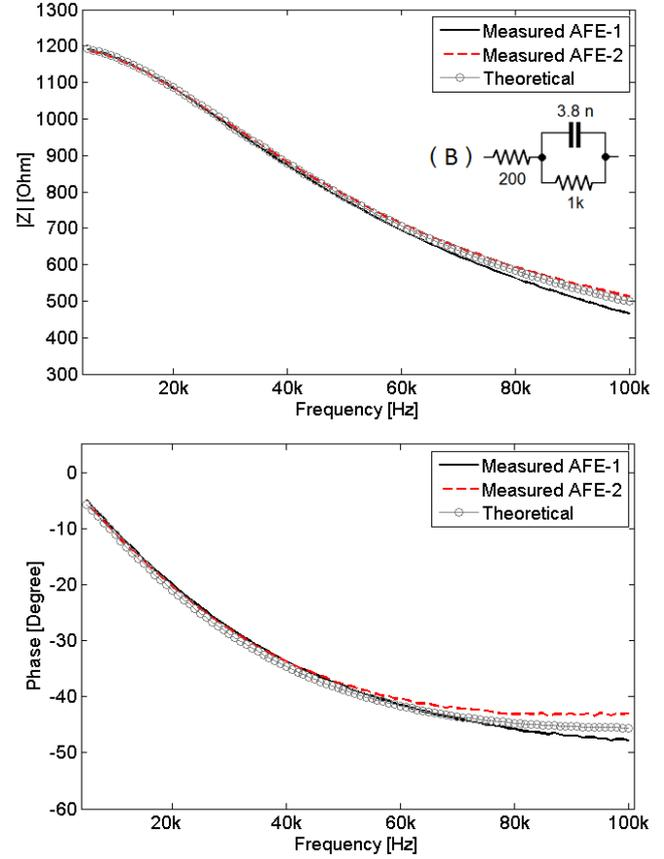
Fig. 5 Frequency response of both module and phase load impedance B.
