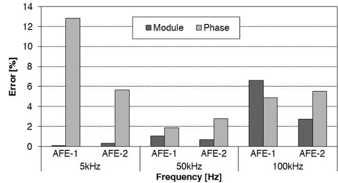
Fig. 6 Error analysis at 3 discrete frequencies for both module and phase load impedance B.
